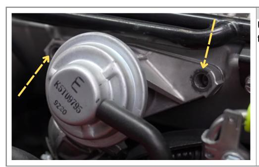
Step 2 Using a 12mm socket, remove the two bolts on the BPV.
