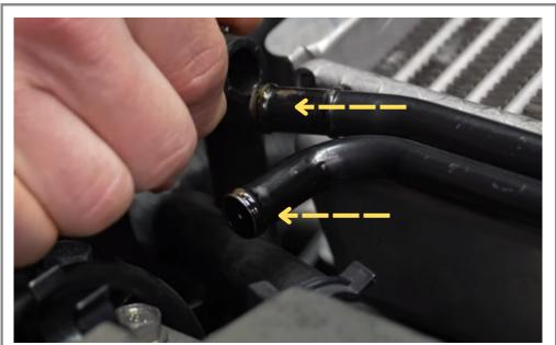
Step 3 Use a pick to loosen the clamps and disconnect the PCV lines.
