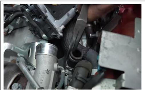
Step 12 **IF** the breather hose does not come off with PCV assembly use a pick to remove the lower clamp.
