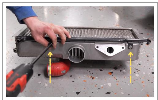
On intercooler use a 10mm socket to remove the two bolts attached to the crossover pipe.
