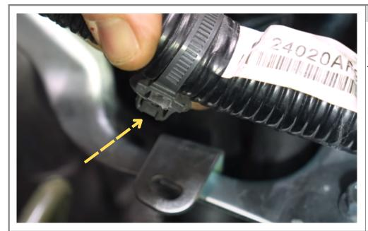
Use needle nose pliers to release the clip that is attached to the wiring harness.
