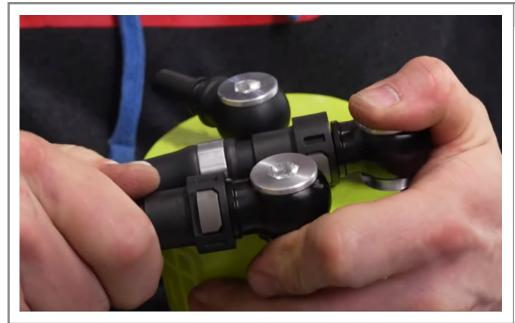
Attach the two 19" coolant lines to the AOS.
