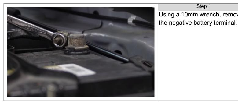
Step 1 Using a 10mm wrench, remove
